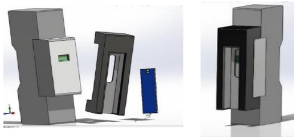
Fig. 4. IR sensor mounting accessory
